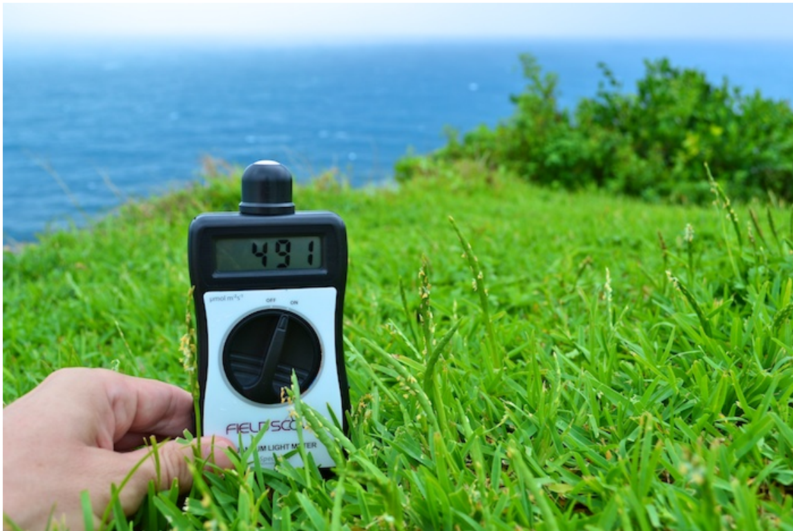
Figure 2: Shown here near Naha, Japan, the quantum light meter from Spectrum Technologies was used to make hundreds of measures of instantaneous photosynthetic irradiance
