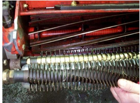
Figure 6 1/4" and 1/2" spacing on groomer reels
