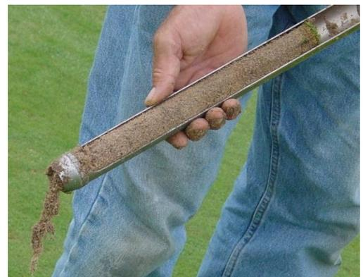
Figure 11. 42 cm soil profile on a 23 year old USGA type green. June 2005, Texas
