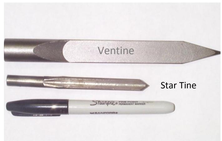
Figure 10. Comparative size of venting tines
