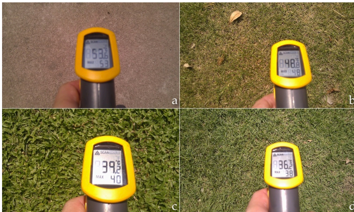
Figure 4: The surface temperature of 4 surfaces at 14:00 on 3 May 2013 in Bangkok when the air temperature was 38°C: a) concrete, 53.6°C; b) wilting Zoysia matrella , 48.8°C; c) transpiring Axonopus compressus , 39.2°C; d) transpiring Zoysia matrella , 36.2°C.
